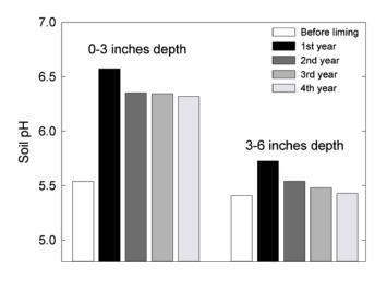
**Figure 2.** Average effect of 3 ton/acre of effective calcium carbonate equivalent (ECCE) on soil pH across four fields managed with no-tillage and corn-soybean rotations.
